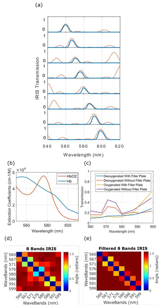
**Fig. 2.** (a) IRIS transmission for the 8-wavelength narrow band system, with filter plate (blue) and without filter plate (red). (b) Oxy (red) and deoxy (blue) hemoglobin extinction coefficients. (c) Transmission of 150  $\mu\text{m}$  quartz capillaries filled with 0% or 100% OS blood using the filter plate (blue) and without filter plate (red). (d) Spectral angle between the 8 IRIS bands. (e) Spectral angle between the 8 IRIS bands using the filter plate.
