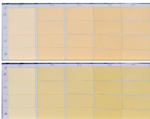
Fig. 2. RGB renderization from hyperspectral reflectance image under two different standard illuminants.
