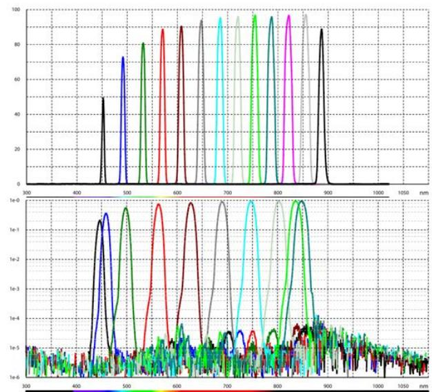
Figure 2: Transmission and blocking characteristics of Continuously Variable Bandpass Filter
