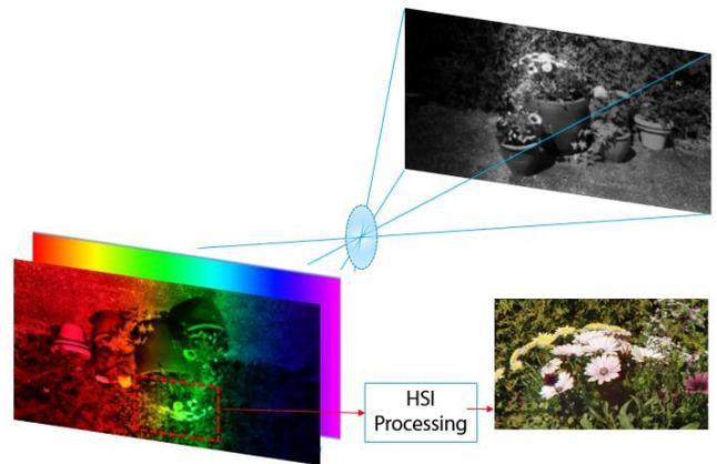
Figure 4: Image acquisition and workflow with filter based Hyperspectral Imaging camera.
