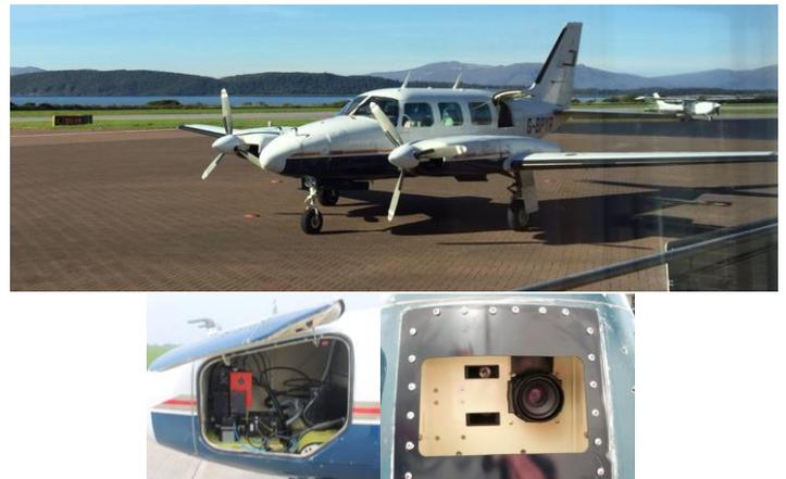
Fig.1 Piper PA-31 Navajo fitted with remote sensing payload
